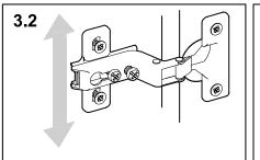
Tighten the screws **D** of all the cross plates.
