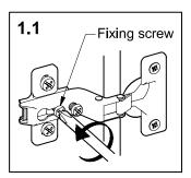
To adjust the door towards the lefthand side - turn the adjusting screw to the right.
