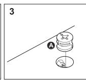
Step 4: Tighten: Turn the cam to the right.
