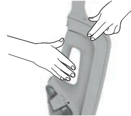
Press the handheld release button and gently pull the handheld from the main body.
