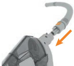
Push the end of the hose with the locking clip into the handheld nozzle until it clicks into place. Make sure the locking clip on the flexi-hose is securely attached by gently pulling the flexi-hose.
