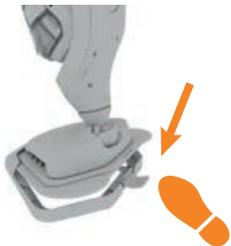
To release the carpet glider, place your foot on clip and push down. Lift steamer to remove.
