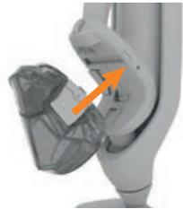
Line up the tank with the machine, push the tank until it clicks into place.
