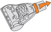
Turn the TurboTool over and slide off the locking ring.
