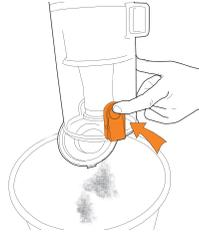
Hold dirt container over a bin and press the dirt container release button to open allowing dirt to fall out.
