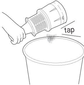
Tap over a bin to remove dirt and debris.
