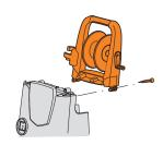
To attach the handle into the top of the pressure washer, align the handle with the screw holes making sure not to trap the solution tube. Slide together and insert 2 screws and turn clockwise to tighten.
