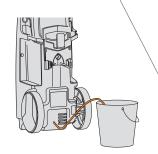
After use rinse the pressure washer to prevent blockages. Inset the solution tube into a bucket of fresh water (Max 40°C), turn the machine on and squeeze the trigger for 1 minute.
