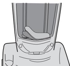
Remove bag door and lift out filter.
