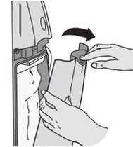
Gently pull bag collar retainer from the hose inlet by pulling off the stiff cardboard at the top of the bag.
