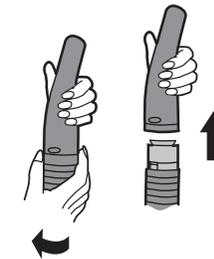
If cleaning tools were in use, check cleaning tool and extension tube first. Next check hose handgrip; to remove grip ribbed ring as shown, turn in direction of arrow and ease apart.
