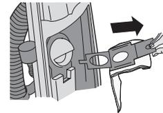
Slide bag from bag collar retainer by pulling on stiff cardboard at top of the bag collar. A shutter will automatically seal off bag opening.
