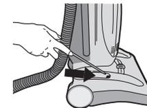
2. Check for a blockage in hose socket. Use a piece of wire or a blunt flexible rod to remove any obstructions.
