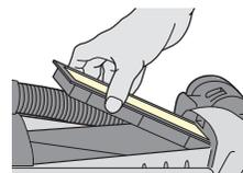
Lift out the exhaust filter.
