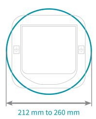
When mounting into glass you will need to cut a hole between 212mm and 260mm in diameter.
