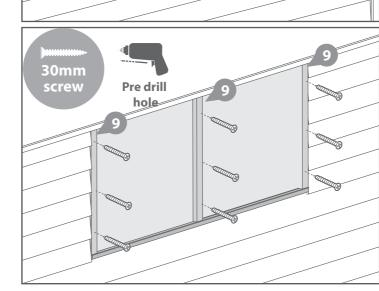
Fix the window strips to the two pieces of framing that sit alongside the outside edges of the window with 3x30mm screws for each strip. **6x30mm Screws**
