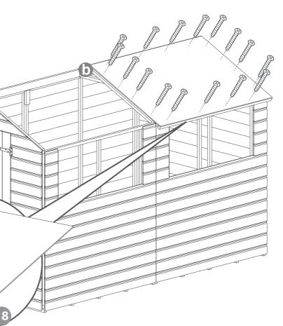
a Fix the eaves frame to the roof sheet using 3x30mm screws for each sheet. 8x30mm Screws
