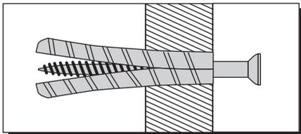
Generally aerated blocks should not be used to support heavy loads, use a specialist fitting in this case.
