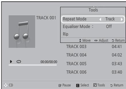
2. To play a particular track, use the ▲▼ buttons on the remote to select the track, and then press the [CD] button.
