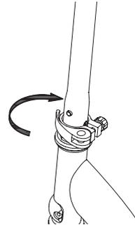
**3** Adjust the tension of the quick release to where you can close the lever all the way to secure the stem.
