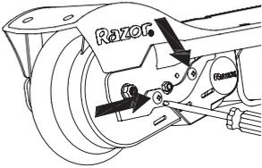
**1** With a Phillips screwdriver, loosen the two screws and remove the chain guard.
