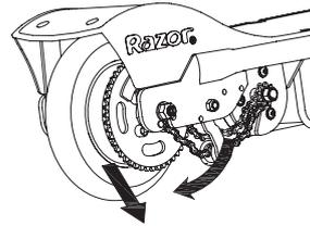
**3** To loosen the chain, push the tensioner down to create some slack in the chain.
