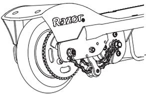
**4** Remove wheel and install replacement wheel. (Note the sequence of the hardware)
