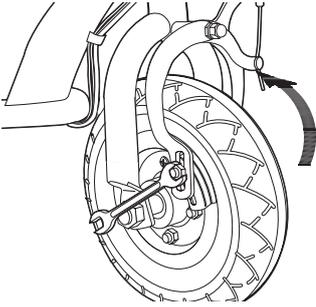
**1** Using a 10mm open wrench, loosen the brake cable bolt.
