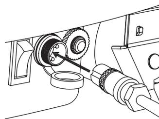
**1** Turn power **OFF** before charging. Plug the charger into the charger port on the electric scooter.
