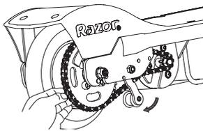
**5** Push the chain tensioner down to install the chain on both sprockets.
