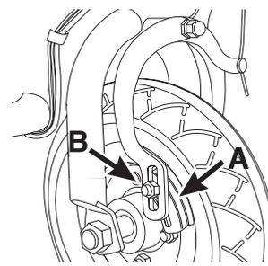
**3** Inspect the brake pads (A) for proper alignment against the wheel or excess wear. To realign brake pads, loosen the fixing nut (B) and adjust the pad to contact the rim. Retighten and test. Readjust as needed.
