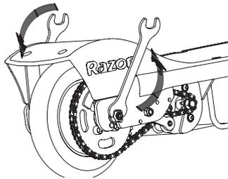
**2** Using two 13mm wrenches, loosen the locknuts by turning the wrenches counter clockwise.
