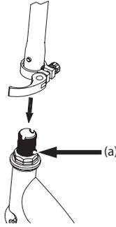
**2** Depress the push button (a) located on the front fork and insert the handlebar stem until the button locks securely into the fork.
