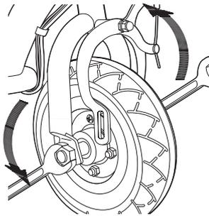
**2** Using two 17mm wrenches, loosen the locknuts by turning the wrenches counter clockwise. Remove wheel and install replacement wheel.
