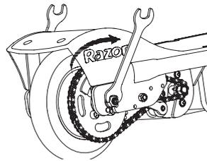
**6** With two 13mm wrenches, re-tighten the locknuts.
