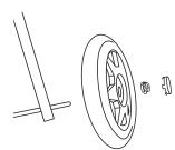
Put the wheels, the plastic ring and the cover on the axes.
