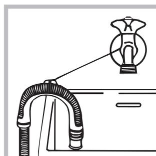
If it is placed over the edge of a basin or sink be sure the free end of the hose is not underwater.
