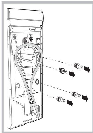
3. Remove the four protective screws and the rubber washer with the respective spacer, situated on the rear of the appliance (see figure).
