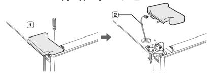
2. Remove hinge screws and the ground screw by turning counter-clockwise, and take off the upper hinge. Be careful that the door does not fall on you as you are removing it
