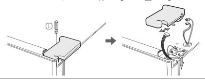
2. Remove hinge screws 2 and the ground screw 3 by turning counter-clockwise, and take off the upper hinge 4. Be careful that the door does not fall on you as you are removing it.
