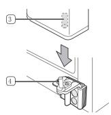
2. Insert the upper hinge shaft 5 into the hole on the hinge 6. Make sure the hinge is level between the upper hinge hole 7 and the hole on the top of the cabinet 8. Then, reattach hinge screws 9 and the ground screw 10 by turning it in a clock wise direction.
