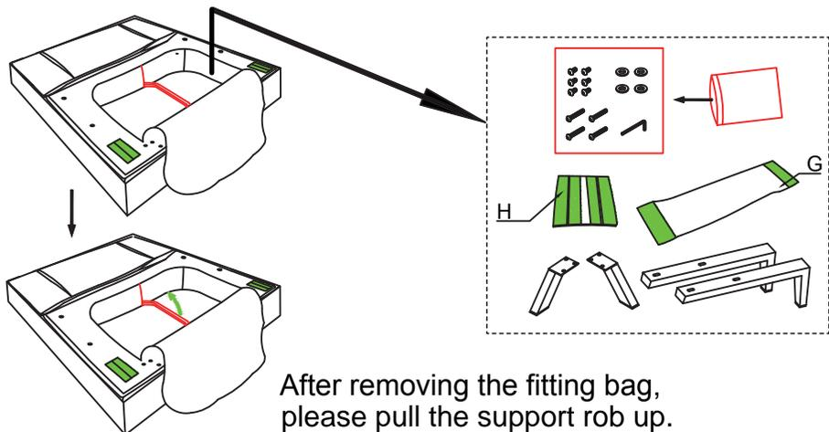
After removing the fitting bag, please pull the support rod up.
