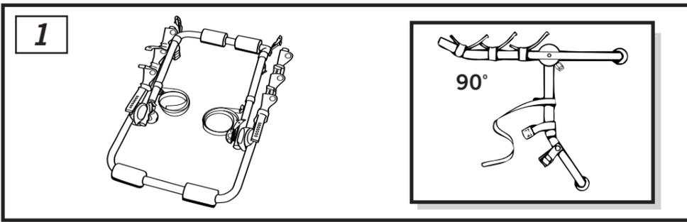
Position the assembled carrier on a clean surface as illustrated. Release the 2 ratchet adjusters and rotate the carrier through 90° and lock in position. The quick release action should be firm for both opening and closing.
