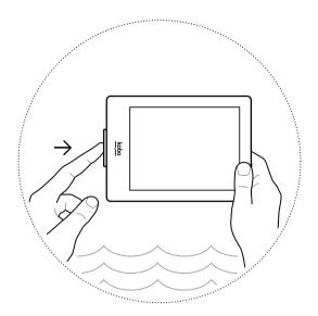
Your eReader has a port cover on the bottom to protect the Micro USB and Micro SD slots from water. To waterproof your eReader, you must close the port cover firmly, as shown in the illustration above. If the port cover isn't firmly closed, your eReader will malfunction if it is submerged in water or used in areas with high humidity, and will no longer be covered by any warranty.
