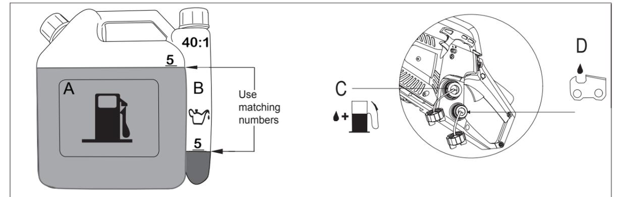
FUEL MIXTURE: 1 Litre (1000 ml) petrol: 25cc (25 ml) 2 Stroke engine oil (40:1 ratio)
