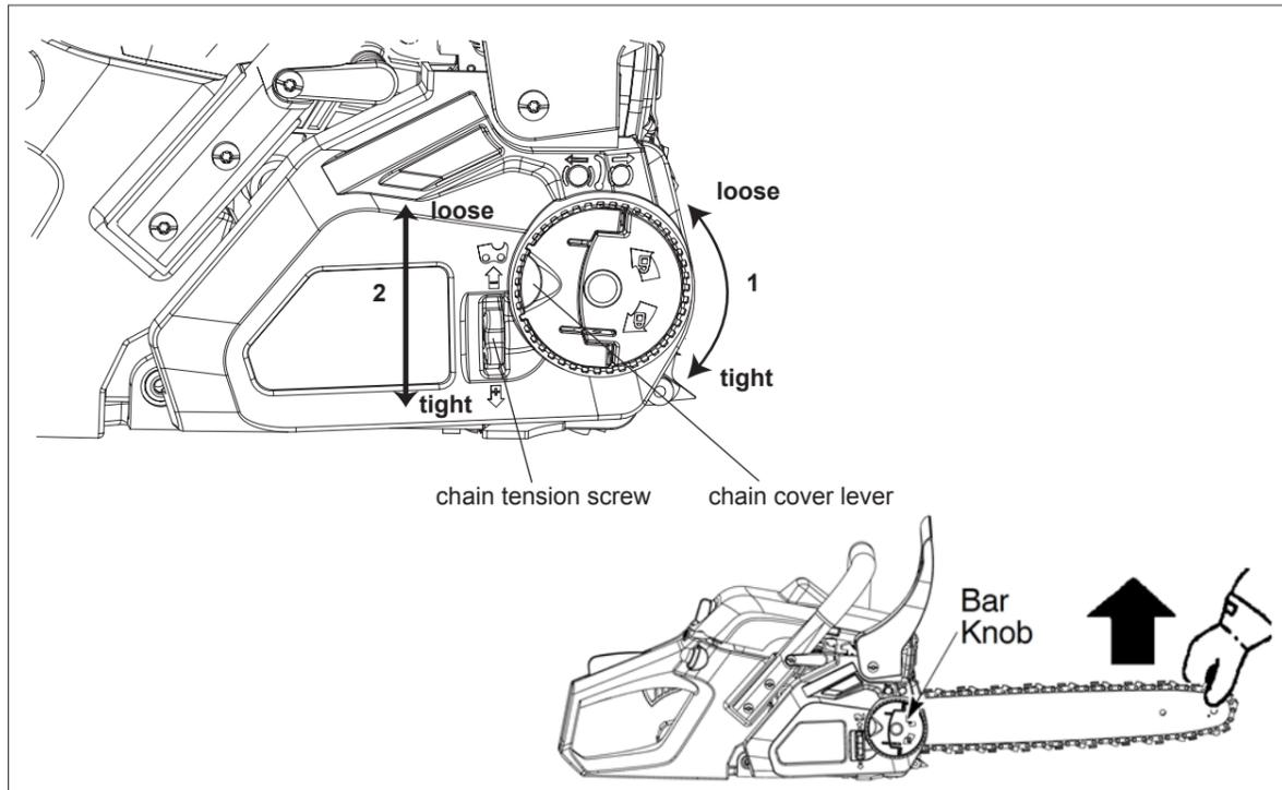
1a Pull the chain cover lever out, and slightly loosen the chain cover.
