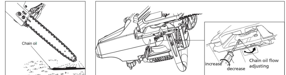
After starting the engine, run the chain at medium speed and see if chain oil is being dispensed as shown.
