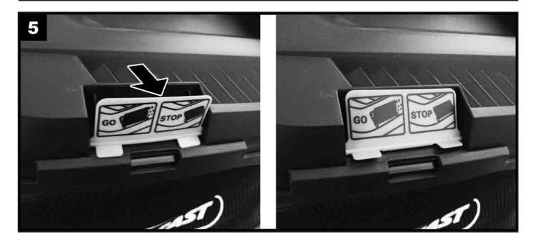
Your mower may be fitted with a grass full indicator. This is a small red flap on the top side of the grass collector.
