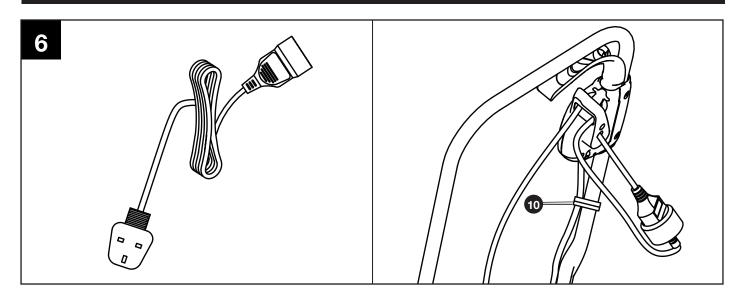
Before you connect the mower to the mains supply make sure that data on the rating plate are identical to the mains data. Connect the plug to an extension cable. It is imperative to sucure the extension cable with the Cable clamp  $\bigcirc$  .
