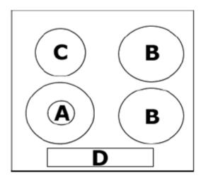
**A** = 3.80 kW triple crown (wok) burner
