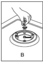
o Unscrew the injector **(B)** and replace it with the stipulated injector for the new gas supply (see table on next page).
