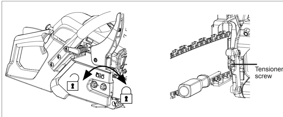
1a Slightly loosen the chain cover nuts.
