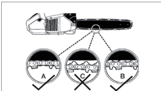
**CAUTION!** If the saw chain is TOO LOOSE or TOO TIGHT the V-drive wheel, chain bar, chain and crank shaft bearing will suffer premature wear. Above fig. shows the correct tension A (when cold) and tension B (when warm). FIG C shows a chain that is too loose.
