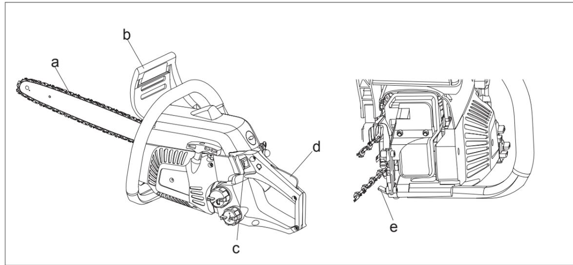
a. **LOW KICKBACK SAW CHAIN:** helps significantly reduce kickback, or the intensity of kickback, due to specially designed depth gauges and guard links.
