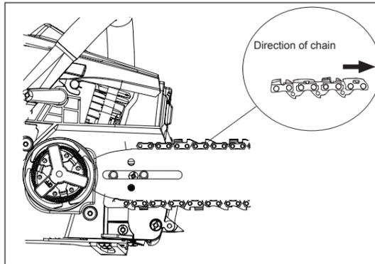
1a Pull the chain-brake back and ensure that it has been released. (the chain cover can only be removed with the chain-brake disengaged)
