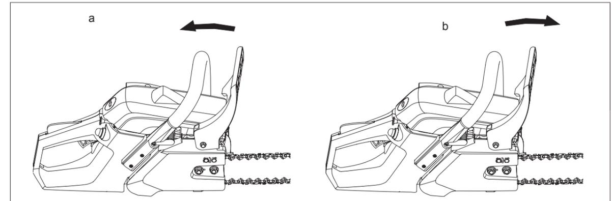
Your chainsaw is equipped with a chain brake that reduces possibility of injury due to kickback. The brake is activated if pressure is applied against the brake lever when, as in the event of kickback, the operator's hand strikes the lever. When the brake is actuated, chain movement stops abruptly.
