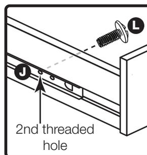
**Note:** Do not overtighten the screws. If they catch on the runner you may need to loosen them slightly.
