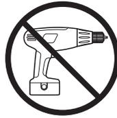
**Warning:** Do not use an electric screwdriver to attach the hinges as this can weaken the fixing.
