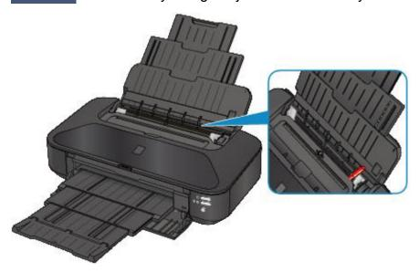
If there are any foreign objects in the rear tray, be sure to turn off the printer, unplug it from the power supply, then remove the foreign object.
