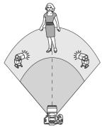
This is convenient when you need a large flash output. All the slave units will fire at the same output and be controlled to obtain a standard exposure.
